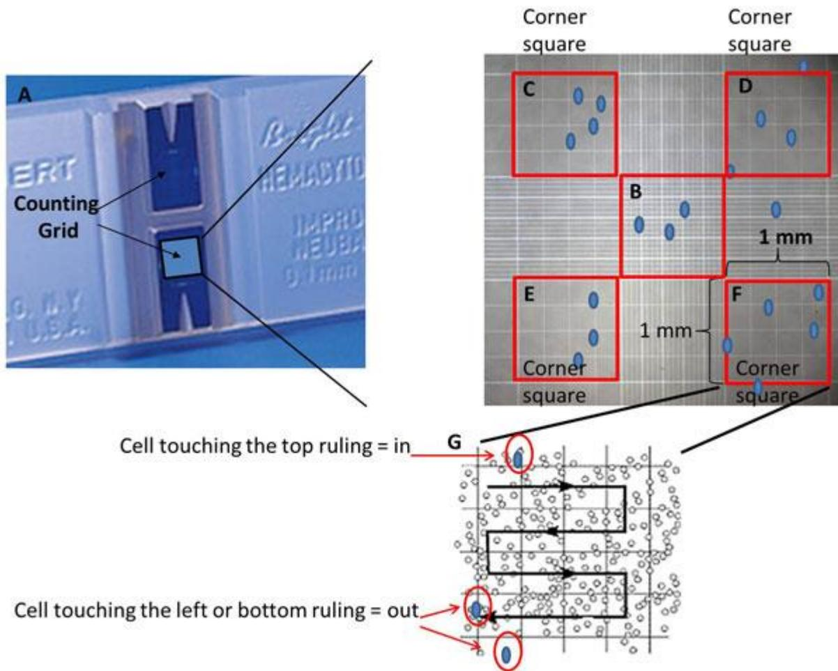
Figure 3. Counting Cells on the Hemocytometer.
